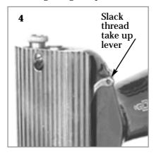
(4) To provide sufficient thread for this loop (not under tension) the thread take up lever on the head travels downwards, rising again to pull the stitch tight.
