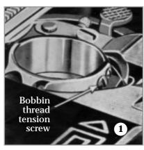
(1) The bobbin has a small spring on its case, which delivers the thread under a slight tension.
