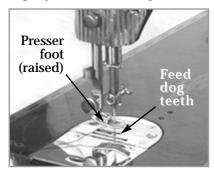
The teeth grip the underside of the cloth and feed it forward a tiny measured amount determined by the setting of the stitch length regulator.
