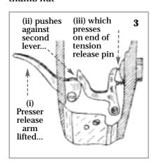
(3) The upper tension is released completely when the presser bar lifter is raised. The lifter presses on a pin which in turn pushes the discs apart.
