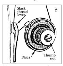
(2) The main tension mechanism is on the upper thread, on the head of the machine.
