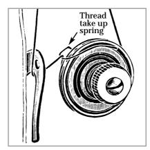
At this point the thread is under extra tension and - to avoid snapping the thread at long stitch lengths - it is passed through the thread take up spring in the tension mechanism which cushions the strain.
